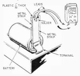
Then solder leads to each metal strip and connect them to your VOM. Insert the lead between the batteries and terminals to make quick current-draw readings.—G. A. WESEN-FELD.
