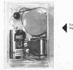
Top view showing high-pressure pushbutton switch.
