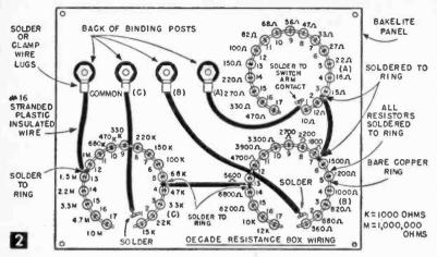
ohmmeter before installing it to make sure that the marked value is accurate to within plus or minus 10% of its markings. When, as occasionally will happen, a resistor is found that is inaccurately marked, substitute another. (If 5% or 1% resistors are used, testing is not necessary. If you are unfamiliar with resistor color coding, an IRC Resist-O-Guide can be obtained for 15¢ from any electronics supply store.) With all resistors sol-
