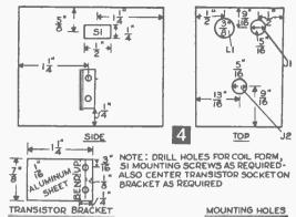
4, mount the coil form (with L1 and L2), input and output jacks (J2 and J1) at one end of the box. Attach the  $\frac{1}{16}$ -in. aluminum transistor socket mounting bracket and "on-off" switch (S1) at the bottom center. Mount B2 vertically next to the transistor and B1 will then fit snugly into the remaining space (Fig. 2).
