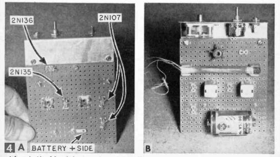
Left, underside of board showing socket and IF transformer terminals prior to wiring. Right, major components mounted on top of board. Spring clip holds battery; fuse clips the antenna coil.
