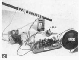
Tuner cambined with powerful sub-miniature, fivetransistor amplifier. All companents can be attached ta the breadboard or installed in an ald radia cabinet.
