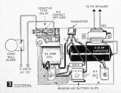
you'll find that voltage applied to the transistor base results in only a tiny flow of current from emitter to collector. By adjusting the spring which controls the armature tension, set the relay so the contacts drop out at about 50 microamperes and pick up at 2 milliamperes. Now if you tune to a station and then tune away from the station's carrier, the relay contacts should close immediately.
