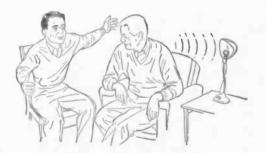
A MICROPHONE stand for hand mikes (such as those that come with less expensive tape recorders) can be improvised from a flexible neck desk lamp with its cord removed (or at least disconnected), a plug to
