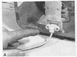
On this set, the cheater cord was originally riveted to the fiber back board. Rivets were removed so the cord could be used as a cheater.
