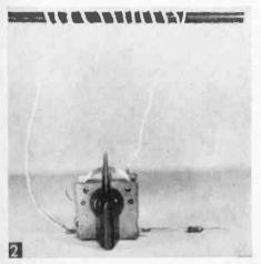
"Triple-C" basic tuner comprises coil, capacitor and crystal.
