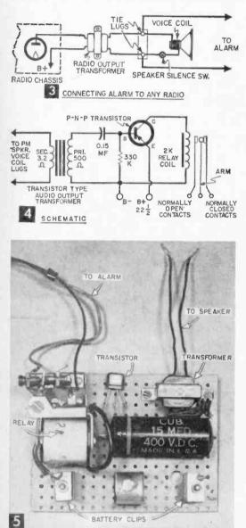
For easy assembly, use a perforated circuit board. Moke the clips of scrap sheet metal.
