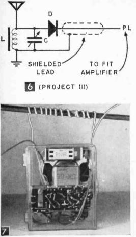
Rear view of crystal diode tuner encased with "Quickie."
