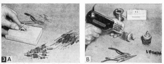
Shape resistor leads around two nails driven in a block of wood to get them of uniform length and with uniform loops (A); then, starting with terminal #1 on each switch with the lowest value resistor, position looped ends of resistors and solder at each terminal (B).
