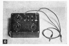
Completed job shows the lettering that was put on with decals sold for the purpose. After decals have thoroughly dried, apply a thin coat of clear plastic with a small brush to make them permanent. Banana plugs and clips soldered to short flexible leads make connections quick and easy.
