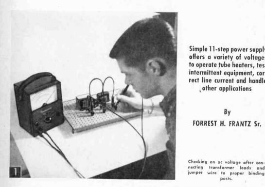
Simple 11-step power supply offers a variety of voltages to operate tube heaters, test intermittent equipment, correct line current and handle other applications
