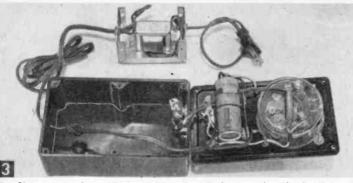
The filament transformer is housed in a small aluminum box (top). Mount the silicon rectifier on an L-shaped aluminum bracket. It is located between the meter and capacitor fastened to the panel with the top switch mounting holes.
