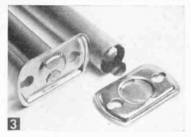
Remove tube flange by prying lugs out with a screwdriver. Do not cut or bend lugs back until pole has been installed in base.
