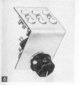
Three-channel crystal selector sub-assembly includes sockets, mounting frame and knob. Right, the threepoint switch installed within a Knight-Kit T-50 amateur transmitter.
