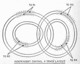
tracks. A 22-gauge solid hookup wire is minimum size for track wiring. Lighter gauge wires on long runs will not feed full voltage
