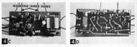
Amplifier after modification, the capacitor having been relocated.
