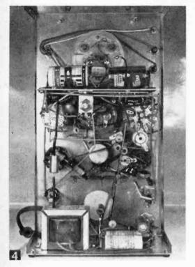
Interior view. Internal transistors are located on small chassis behind batteries.
