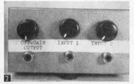
Closeup view showing input and output jacks.
