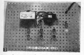
Parts mount easily on a perforated board.
