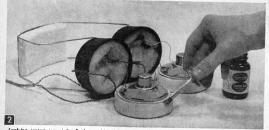
Applying contact cement for final assembly. The earphone housings, made of plastic cups, are filled with a backing of fiberglass to eliminate stray sounds back of the speaker cones.
