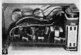
Amplifier completely assembled with battery tucked in place.
