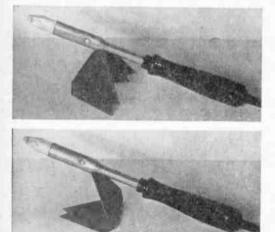
• You can stand or toss this temporary soldering iron rest onto the bench, and use it in whatever position it comes to rest. Shaped like
