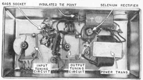
All wiring is under the chassis. Six holes just above the output tuning circuit on this photo feed input, output and power leads through to a 6-terminal barrier strip on top.
