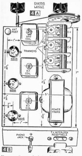
Your capacitor may be designed for horizontal operation. There is ample room on the chassis for either mounting.
