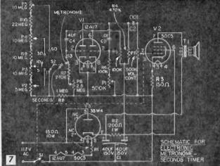
**Calibration is Next**, after a wiring check. Turn S3 to "seconds" and S2 to the onesecond position. Turn the unit on with volume about half way up. You should hear ticks from the speaker in about 30 seconds. Allow a ten minute warm up period, and then use an electric clock second hand to adjust pot P1 until the click frequency is exactly one per second. Pot P1 is left in this position throughout the rest of the calibration.
