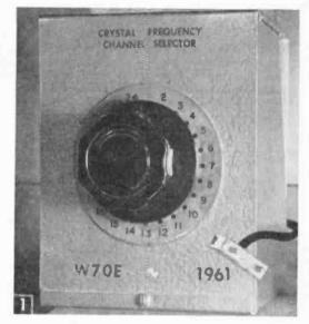
External 24-channel crystal frequency selector fitted with coaxial cord and plug to fit crystal socket in the transmitter.
