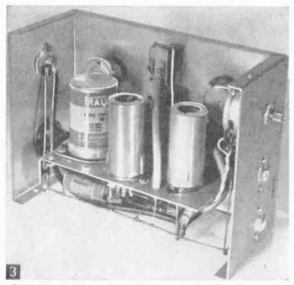
Back of panel view of mixer with cover removed. Note Input jacks and Hum Control on end panel at right.
