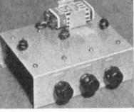
pending on make and type — for such operation.) Because of the low output of magnetic cartridges, a device known as a preamplifier is usually employed with them to effect the desired boost. The preamplifier is connected between the cartridge and the power amplifier in a simple plug-in circuit.
