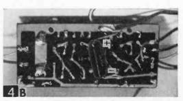
Amplifier before modification with original position of 30 mfd, 10 volt capacitor to be relocated.
