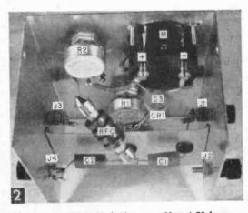
Aluminum baffle shields bridge arms C1 and C2 from the rest of the circuit to prevent interaction at high frequencies. Binding posts J2 and J4 are grounded to the cabinet, while J1 and J3 are insulated with extruded washers.
