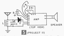
plifier to the switch (S) and the black, yellow, and green leads to the volume control (R1). Connect the black lead to the low volume end lug and the yellow to the center lug.
