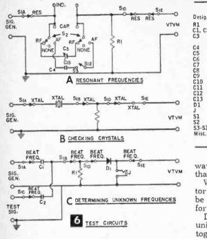
frequency. The amount of rise in voltage gives an indication as to the activity of the crystal. Its harmonic content can also be checked by tuning the signal generator to the crystal's harmonic frequencies.
