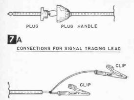
With this test lead you can trace signals in the audio portion of radios, audio amplifiers, and other low frequency radio equipment. You can also test microphones, phonograph pick-ups, vibration transducers, and other "energy changers." When you use it as a test amplifier, connect the test lead shield to ground and the center lead to the high point in the unit under test.
