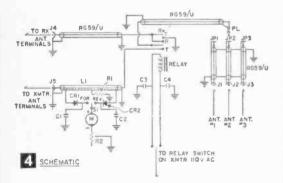
out a similar hole punched in the other end of the shield. Insert the insulated center conductor and spread the shield tight again. Wrap the shield ends with bare wire and solder to hold it in place. At midpoint from where the hookup wire enters and leaves the coax, spread the shield and pull a couple of inches of hookup wire out for connection of R1.
