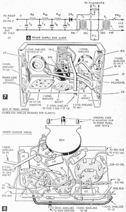
(the one being heard) position, and switch the Function Switch to "Fade." The second signal will still be grounded by the Transfer Switch and the first signal will still be connected directly to the grid of V2—but through the Fader Control at zero resistance. When desired, turn the Fader
