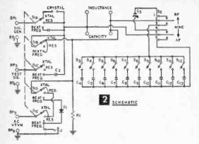
cies. At high radio frequencies, the internal capacity of the unit becomes important because of the low capacities. In such case, a smaller variable capacitor (100 or 140 mmfd) should be used. In addition, you would have to minimize internal capacity by placing parts and controlling lead length in a more careful manner.
