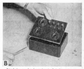
Attach the completed panel to the Bakelite meter case, using 4-40 screws at the four corner holes (B). It fits flush in recess of case.
