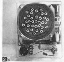
View showing holes drilled for speaker sound.
