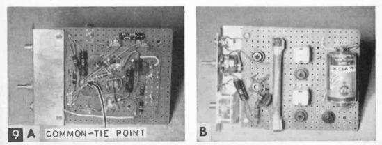
For a good wiring job, keep capacitors and resistors close to board and use spaghetti tubing an leads crossing bare leads or terminals to avaid shorts. Right, transistors shown in sockets on top of board where wiring is limited.
