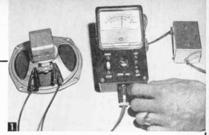
Low range on most ohmmeters is 0 to 1,000 ohms. This meter gives you dependable readings of low ohmage parts such as this speaker coil. You can calibrate the meter to read even in fractions of an ohm.
