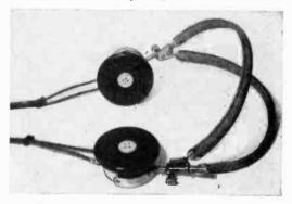
the diaphragm is protected from damage by sharp objects when phones are stored or transported. The button also provides a better earseal between the cap opening and the eardrum. -A. TRAUFFER.
