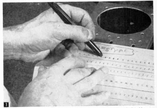
Transfer letters are applied by laying the sheet an the panel and rubbing the back of the desired letter.
