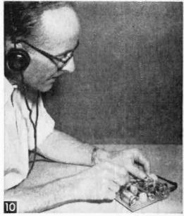
Listening in on an antenna trimmer adjustment, ane af several steps in aligning the set.
