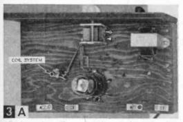
Ferrite tuning coil mounted through chassis is subject of many experiments conducted with temporary "hank" form coils.
