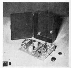
Two spacers cut from pipe are cemented to back of case to hold board in proper position.
