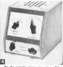
On the seconds range, you get a click every 1, 5, 10, 30, or 60 seconds. Each range has its own control pot on the back of the chassis for calibratian.
