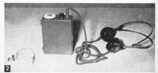
Side of plastic case is actually top of the set, where all controls are located for convenient operation.
