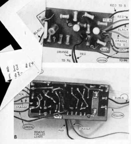
Top view of printed circuit amplifier showing colored leads. Be sure to read instructions packed with this board.
