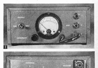
This convenient unit selects antennas, measures efficiency, and switches the antenna from receiver to transmitter.
