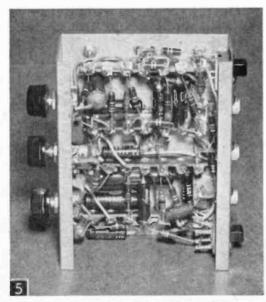
Completely wired chassis, bottom view.
