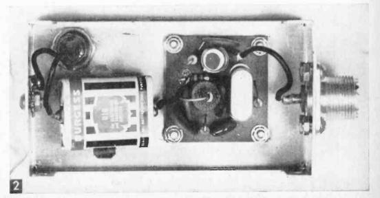
Underview shows printed circuit module and battery.
