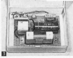
The complete circuit fits in a 4-in.-long plastic box. A single hearing aid battery provides 22½-volt power.
