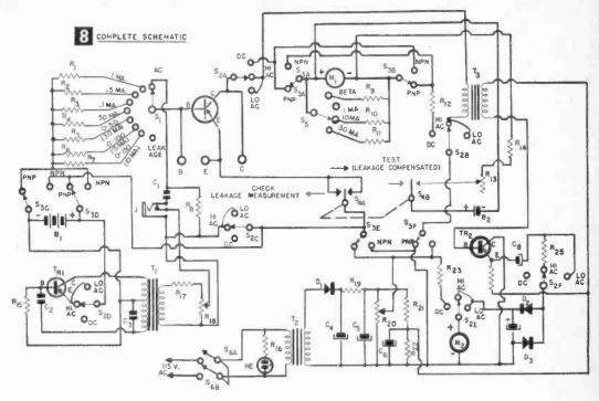
Move test switch to "test" and read net beta on appropriate scale of meter M1.
